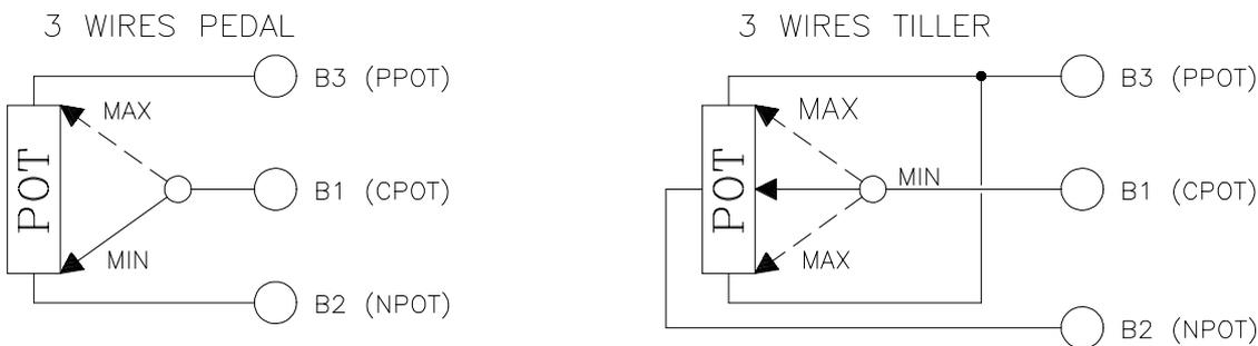
Automatic minimum and maximum signal acquisition must be carried out (PROGRAM VACC function) using the programming console and in both directions. This function is indispensable when compensating an eventual asymmetry in the mechanical components of the potentiometer and for minimum level adjustment in particular.
