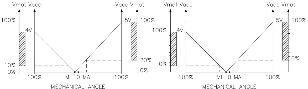
The above graphs show the output voltage of a potentiometer that has not been calibrated compared to the mechanical “zero” of the tiller knob (MI and MA indicate the closing points of the microswitches, 0 represents the mechanical angle of rotation of the throttle). The first graph shows the corresponding motor voltage without acquisition; the second graph shows the corresponding voltage after potentiometer signal acquisition.
